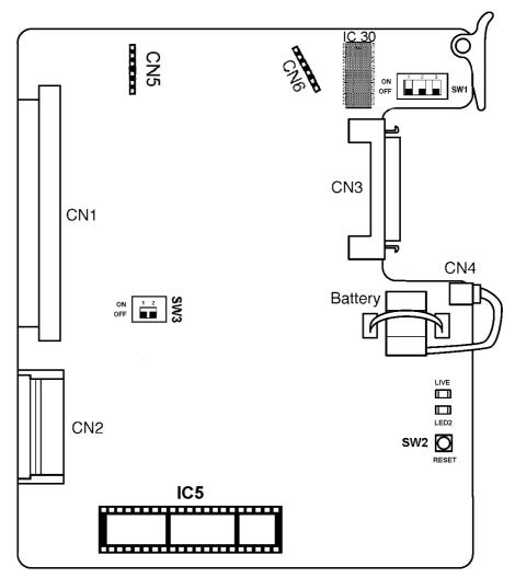
Figure 2-2: CPUI( )-U( ) ETU Switch Settings
